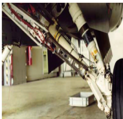
图24 F-16主起落架下部支撑杆 Fig.24 Lower-after poles of main landing gears of F-16 fighter
